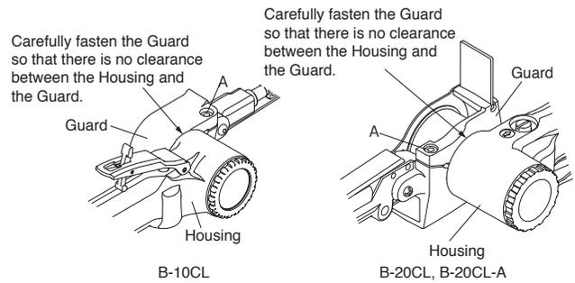
Carefully fasten the Guard so that there is no clearance between the Housing and the Guard.
